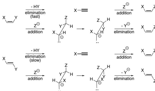
**Scheme 1.** Elimination–addition versus addition–elimination in nucleophilic substitutions on vic-disubstituted ethenes.
